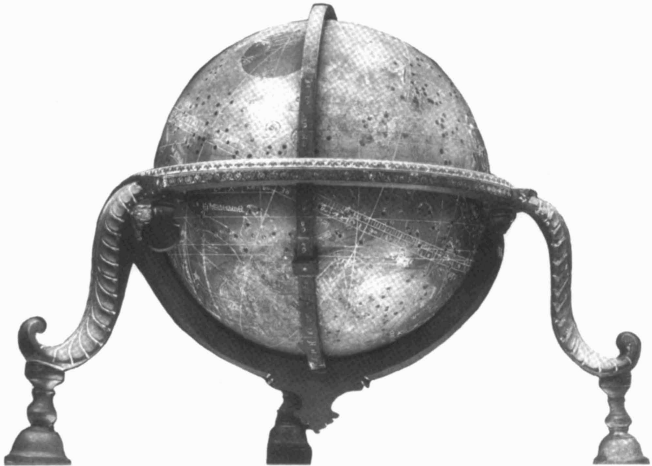
FIG. 2.31. ISLAMIC CELESTIAL GLOBE, UNSIGNED AND UNDATED, ENGRAVED IN SANSKRIT, DEVANAGARI SCRIPT. The sphere is a hollow seamless sphere cast by cire perdue . It is a product of the workshop of Lālah Balhūmal Lāhūri, who was active in Lahore in the first half of the nineteenth century.
