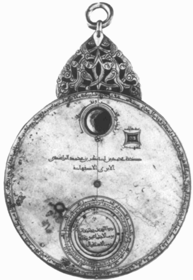
FIG. 2.17. REVERSE SIDE OF THE ASTROLABE SHOWN IN FIGURE 2.16. The phases of the moon are displayed through the circular window near the top of the instrument. Two circular plates beneath, one with a disk for the sun and the other with a disk for the moon, rotate within a zodiacal calendar. Diameter of the original: 18.5 cm. Museum of the History of Science, Lewis Evans Collection, Oxford (inv. no. IC5). By permission of the Bettman Archive, New York.
